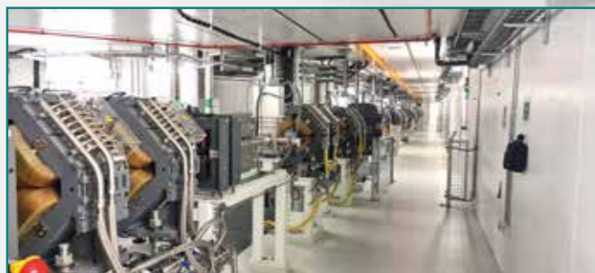
The protons are accelerated to 2/3 of the speed of light before they are directed into the beam line behind the treatment rooms.
