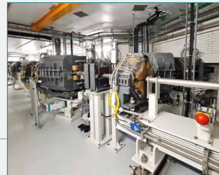
The beam line directs the protons from the accelerator to the treatment rooms. Magnets bend and focus the beam. Photo: Danish Centre for Particle Therapy
